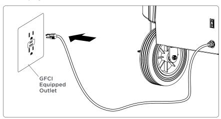
**NOTE:** A live power outlet can be verified when the Power Breezer is **plugged in and powered off** by pressing the **oscillation** or **water buttons.** The LED lights will dimly illuminate when either of these buttons are depressed.
