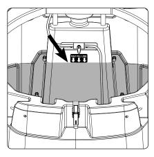
Do not fill the water tank above the max fill level, as shown. If water tank is filled past this level, water may leak out of the water tank and cause a hazard around the Power Breezer.
