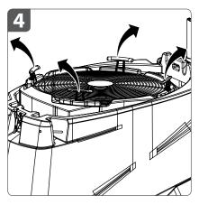
**4.** Tilt up the four **fan head handles**, if they are folded down, prior to lifting the head.
