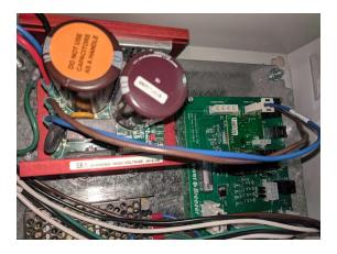
• Verify that the AC Drive is receiving the correct voltage. Check the VFD Power output (H3) for 120VAC.
