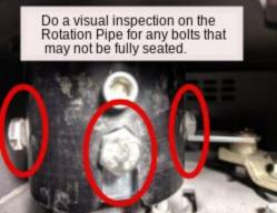
2. Inspect the Rotation Linkage for any signs of defect or loose bolt. This can also cause the Head to rotate erratically.
