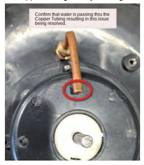
Check the Atomizer for water before reassembling
