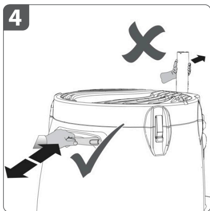
When moving Cooling Unit, be sure to use the transport handle and not the head support pole .
