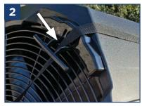
Feed each of the (4) tie straps through the head's handles as shown.
