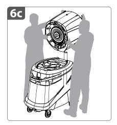
6c. Once again, lift the fan head and align it with the fan head support pole. Once the fan head is seated on the fan head support pole, rotate the fan head horizontally until you feel it engage with the fan head support pole.
