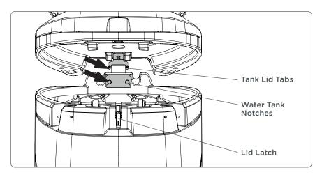
Note the lid tabs on the back underside of the lid.
