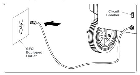
**NOTE:** A power outlet can be verified that it is functioning when the Power Breezer is plugged into it. If functioning, the **Circuit Breaker** on the Power Breezer will illuminate. If the **Circuit Breaker** does not illuminate:
