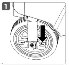
Before you get started, be sure to lock both of the rear wheels by pressing down on the brake lever to set them to the ON position.
