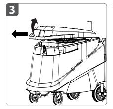
**3.** Remove **tank lid** by first lifting up on the **transport handle** and then pulling forward.
