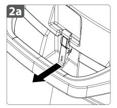
2a. Open the lid latch by first pulling forward the lower portion of the latch.2b. Finish opening the lid latch by pulling the upper portion of the latch forward and away from the lid.
