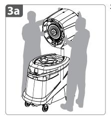
**3a.** Lift the **fan head** straight up and off the **head support pole**.
