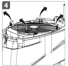
4. Tilt up the four **fan head handles**, if they are folded down, prior to lifting the **head**.
