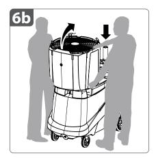
**6b.** Both people should re-adjust their grip so that they have one hand on a **fan head handle** or the black outer housing and one hand on the front edge of the **fan head**, as shown.
