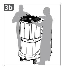
**3b.** Carefully rest the **fan head** on the **edge of the tank**.
