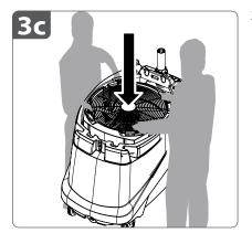
**3c.** Carefully lower the **fan head** into the **water tank**.
