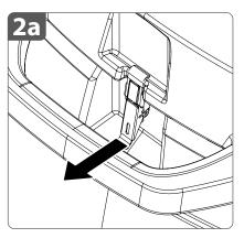
**2a.** Open the **lid latch** by first pulling forward the lower portion of the latch.**2b.** Finish opening the **lid latch** by pulling the upper portion of the latch forward and away from the lid.
