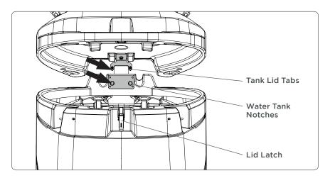
Note the tank lid tabs on the back underside of the tank lid.
