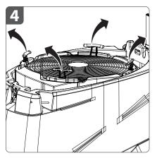
Tilt up the four fan head handles, if they are folded down, prior to lifting the **head**.
