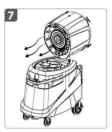
Once installed, the **atomizer** (metal disk) will be facing the **water tank**, air will be blown *over* the **water tank** when the Power Breezer is turned on.
