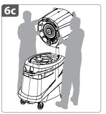
**6c.** Once again, lift the **fan head** and align it with the **fan head support pole**. Once the **fan head** is seated on the **fan head** support **pole**, rotate the **fan head** horizontally until you feel it engage with the **fan head support pole**.
