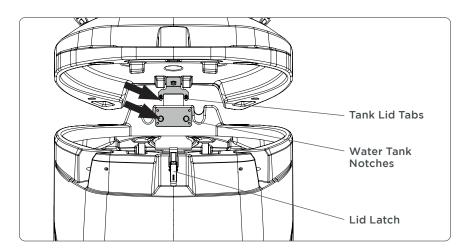
Note the lid tabs on the back underside of the lid.
