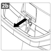
**2b.** Finish opening the **lid latch** by pulling the upper portion of the latch forward and away from the tank lid.
