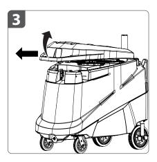
3. Remove tank lid by first lifting up on the **transport handle** and then pulling forward.
