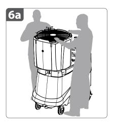
**6a.** Lift the **fan head** straight up and out of the **water tank**. Carefully rest it on the **edge of the water tank**.
