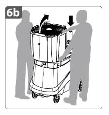
**6b.** Both people should re-adjust their grip so that they have one hand on a **fan head handle** or the black outer housing and one hand on the front edge of the **fan head,** as shown.
