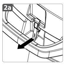
**2a.** Open the **lid latch** by first pulling forward the lower portion of the latch.
