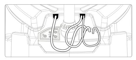
**2a.** Route the fan **head power cord, atomizer drain hose, and water inlet hose** through the openings in the back of the **water tank** as shown above.
