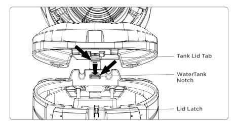
Note the tank lid tab on the back underside of the tank lid.
