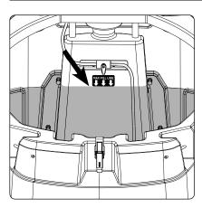
Do not fill the water tank above the max fill level, as shown. If water tank is filled past this level, water may leak out of the water tank and cause a hazard around the Power Breezer.
