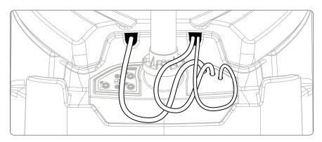
**4a.** Route the fan **head power cord, atomizer drain hose, and water inlet hose** through the openings in the back of the **water tank** as shown above.
