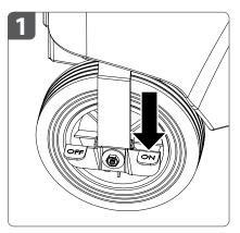
1a. Before you get started, be sure to lock both of the rear wheels by pressing down on the brake lever to set them to the ON position.
