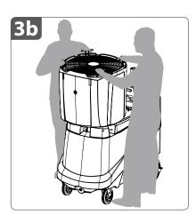
**3b.** Carefully rest **fan head** on the **edge of the tank** opposite of the **head support pole**, as shown.
