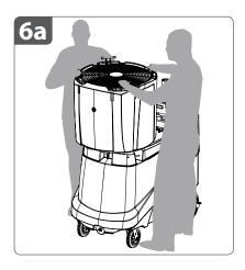
6a. Lift the fan head straight up and out of the water tank. Carefully rest it on the edge of the water tank opposite of the fan head support pole, as shown.
