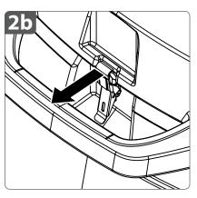
**2b.** Finish opening the **lid latch** by pulling the upper portion of the latch forward and away from the lid.
