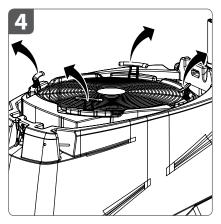
**4.** Tilt up the four **fan head handles**, if they are folded down, prior to lifting the head.
