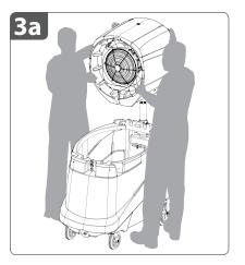
**3a.** Lift the **fan head** straight up and off the **head support pole.**
