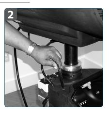
Remove water inlet hose from the front hole in the tank.
