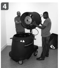
Once installed, the **atomizer** (metal disk) will be facing the **tank**, air will be blown *over* the **tank** when the unit is turned on.
