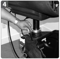
Store the water **inlet hose** in the front hole on top of tank, from where atomizer drain hose was removed.
