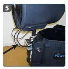
Once assembled, the **drain hose** should be flexible, but not so loose that water gets backed up in the hose.
