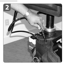
Take **atomizer drain hose** out of the front hole on top of the **tank**.
