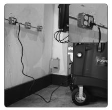
For safety, only plug your unit into outlets equipped with GFCI. **DO NOT plug into standard outlet** without a GFCI feature.
