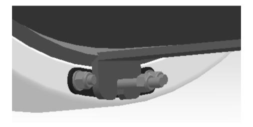
14. Tighten the top and bottom M8 nuts until the gap between the Shroud and the Sound Dampener has closed.
