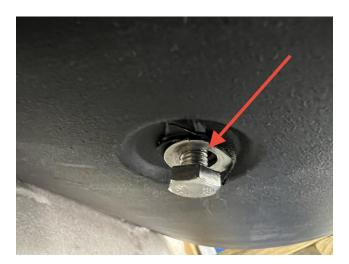
8. Attach the Mohawk Lock Bracket (150-302-444-1) to the shroud through the keyhole.
