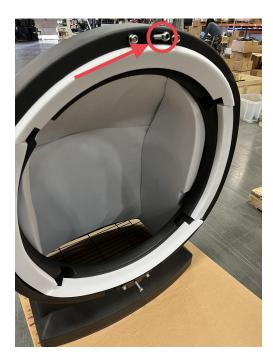
12. Hang the Sound Dampener Assembly to the Saddle Lock Bracket as shown below.
