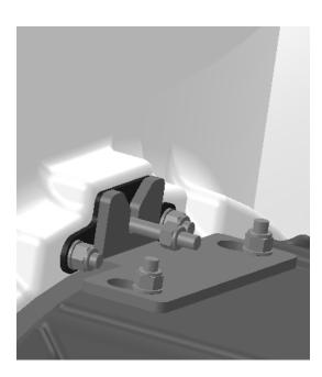
13. Re-insert the M8 nut you took out from Step\_11 to the bottom of the Sound Dampener Assembly through the Mohawk Lock Bracket.
