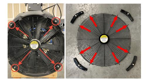
4. Loosen the rear top two M8 saddle nuts until you have 1/4in clearance with two 13mm socket wrenches (one holds the saddle bolt inside the shroud and one loosens the M8 nut).
