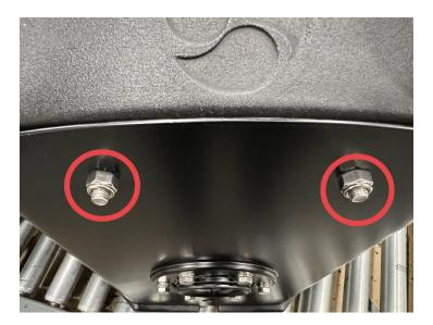
5. Attach the Saddle Lock Bracket (150-302-439-1) to the saddle through the keyholes.
