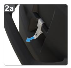
**2b.** Finish opening the **lid latch** by pulling the upper portion of the latch forward and away from the **tank lid**.
