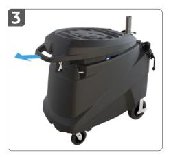
**4.** Tilt up the four **fan head handles**, if they are folded down, prior to lifting the **fan head**.
